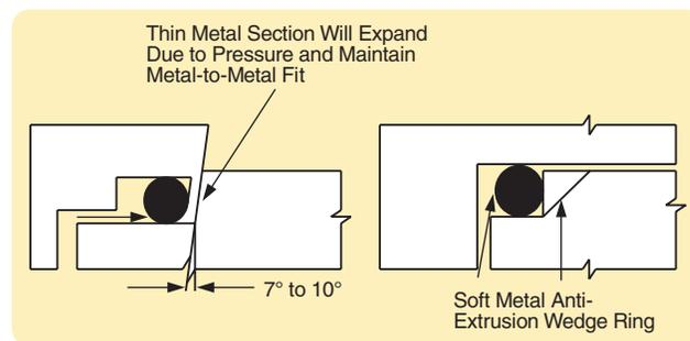
Figure 6-2: Clearance Control for High Pressure Seals
