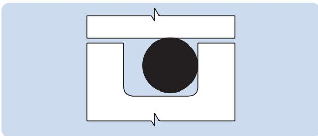
Figure 5-19: Floating O-Ring Seal
