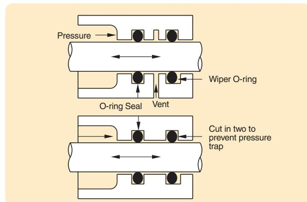
Figure 1-14: Wiper Installation
