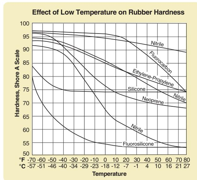
Figure 2-18: Effect of Low Temperature on Rubber Hardness
