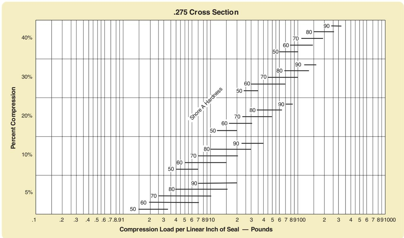
Figure 2-8: .275 Cross Section
