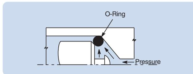
Figure 5-23: O-Ring Blow-Out, Standard Groove
