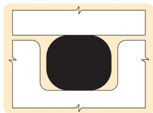
Figure 1-4: O-Ring Installed
