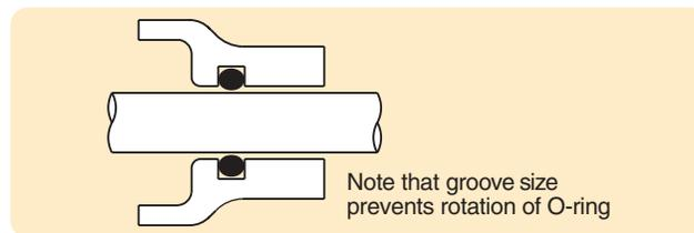
Figure 1-11: Rotary Seal
