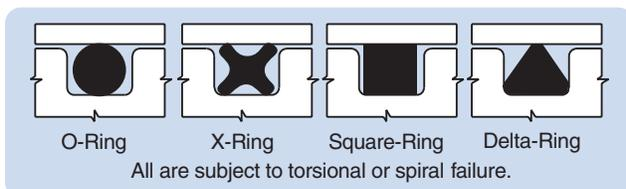
Figure 5-17: Ring Cross-Sections for Reciprocating Seals
