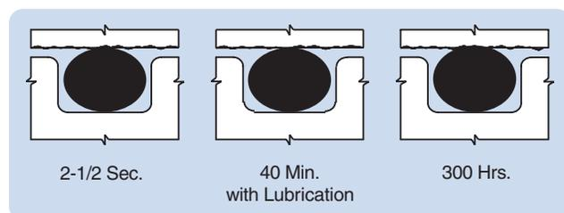
Figure 5-8: Flow of O-Ring into Metallic Surfaces
