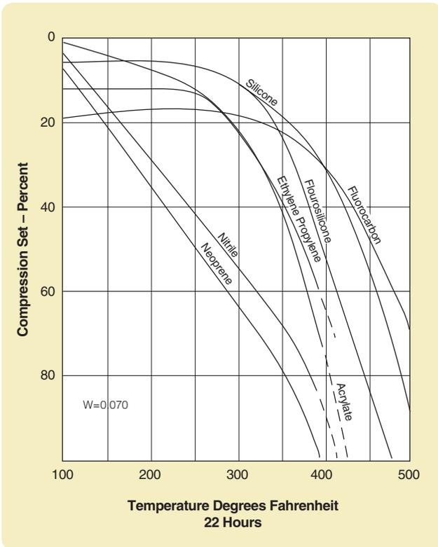
Figure 2-14: Compression Set .070 Cross Section
