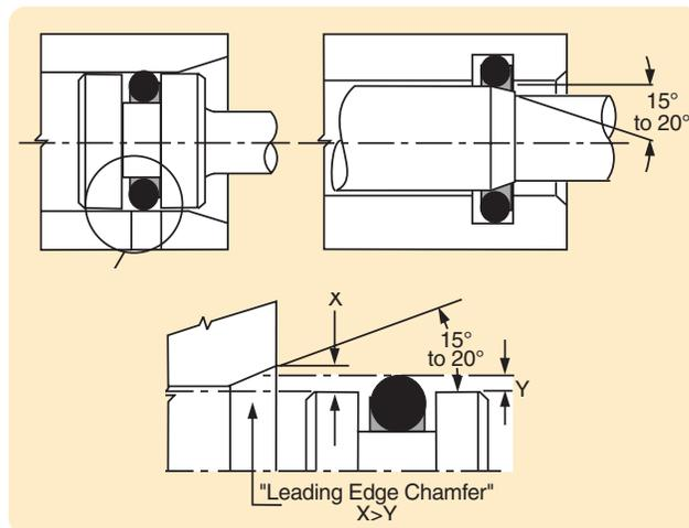
**Figure 10-6: Chamfers**
