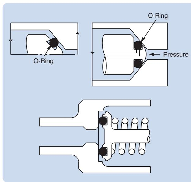
Figure 5-24: Groove Designs to Prevent Blow-Out
