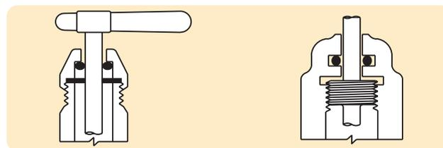
Figure 1-10: Oscillating Seal
