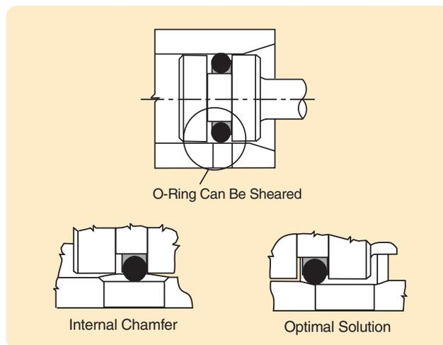
**Figure 10-7: Drilled Port Assembly**
