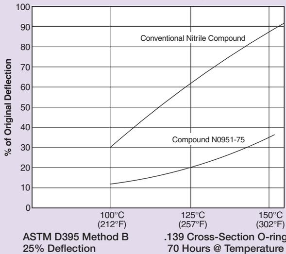
**Figure 3-7: Compression Set Resistance of Compound N0951-75**
