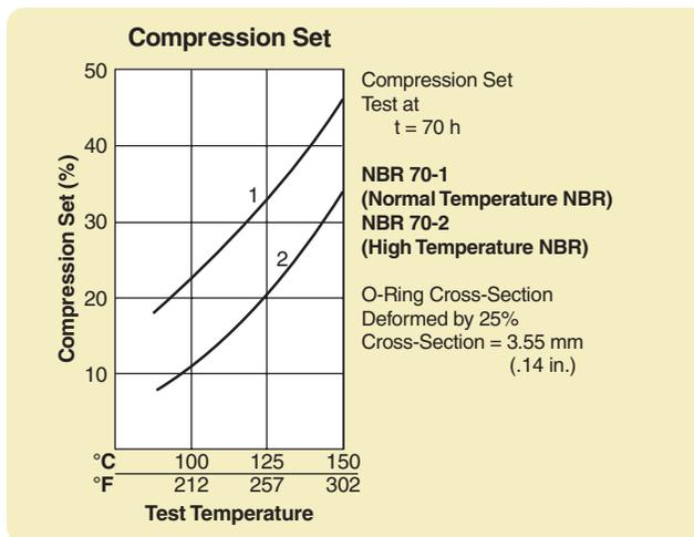
Figure 2-12: Compression Set vs. NBR 70 Compounds
