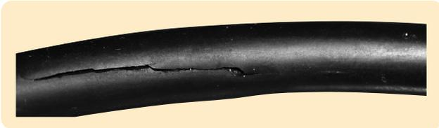
Figure 10-4: O-Ring Damaged by Explosive Decompression
