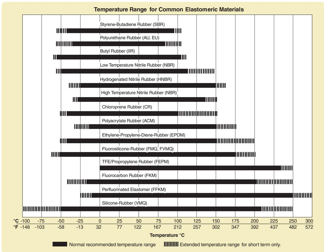
Figure 2-3: Temperature Range for Common Elastomeric Materials
