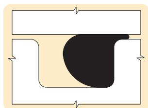
Figure 1-6: O-Ring Extruding
