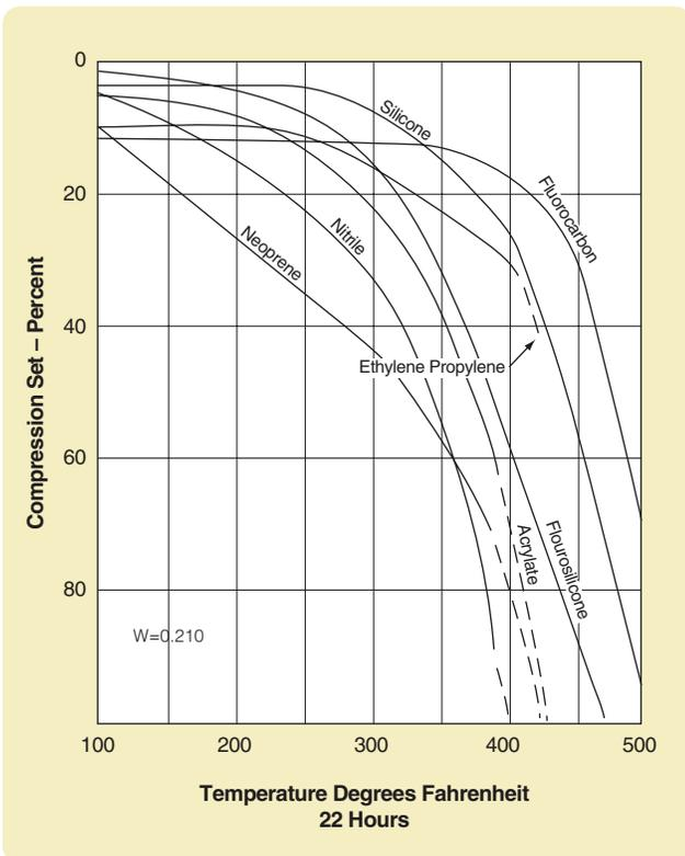
Figure 2-16: Compression Set .210 Cross Section
