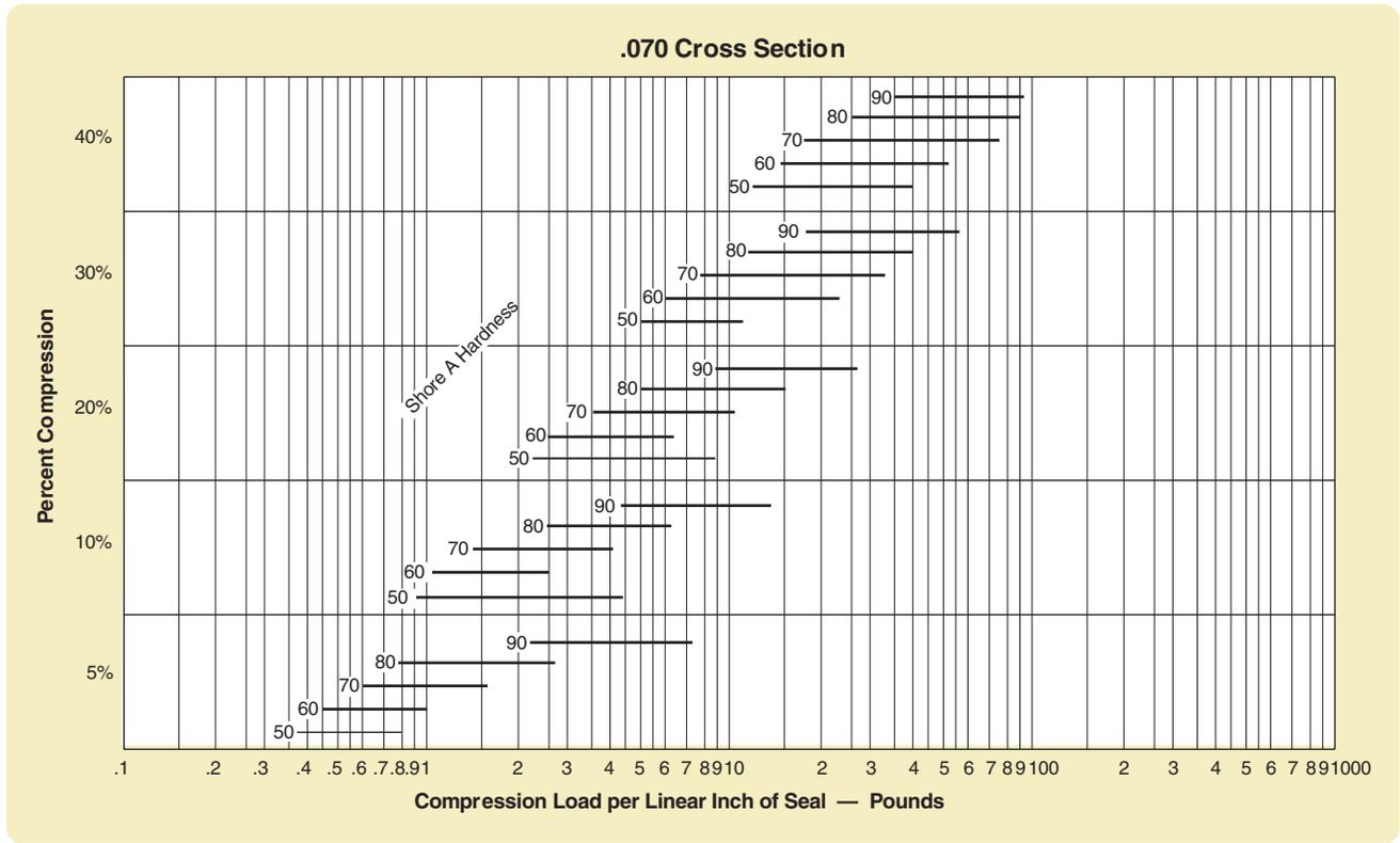
Figure 2-4: .070 Cross Section
