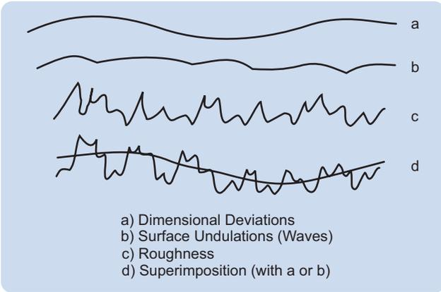
Figure 5-3: Surface Finish Structure
