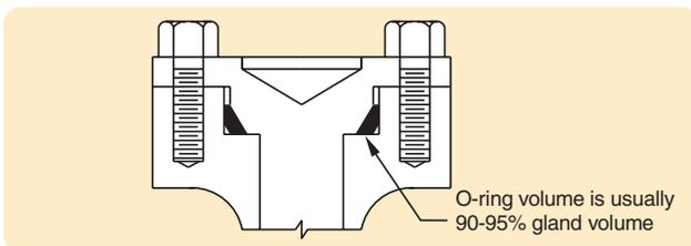
Figure 1-13: Crush Installation
