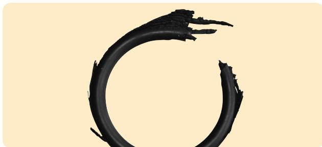
Figure 10-2: Extruded O-Ring
