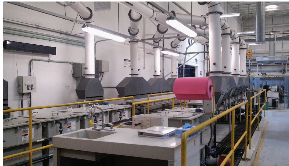
Parker Chomerics integrated chemical conversion coating (chem-film) manufacturing line.
